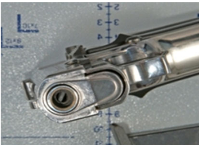
FIG. 3—Appearances of the barrel obstruction.
