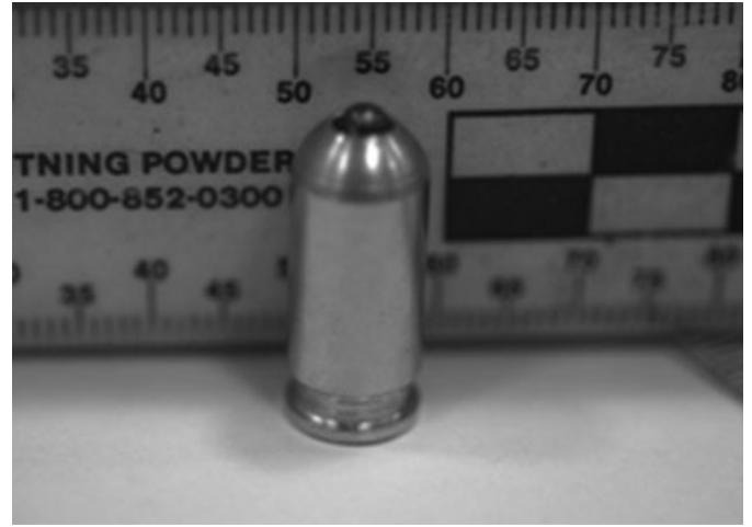
FIG. 4—Different type of modified blank cartridge fitted with buckshot.
