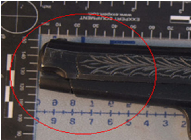
FIG. 10—Cracking of the barrel due to the higher pressures generated from firing a conventional cartridge.
