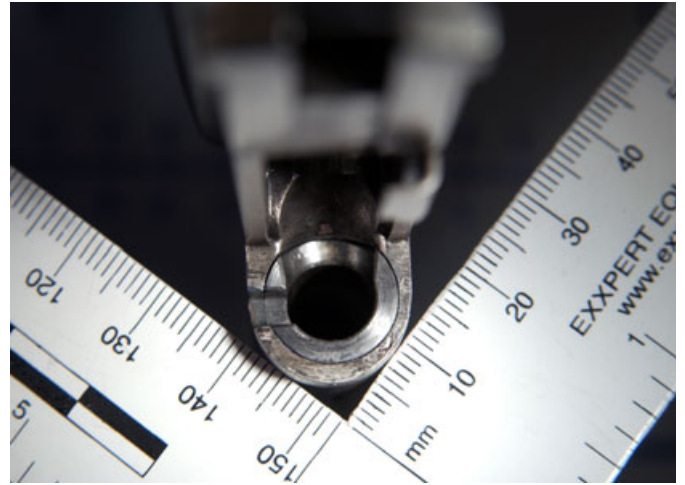
FIG. 8—Sleeving a narrower tube into an original barrel.
