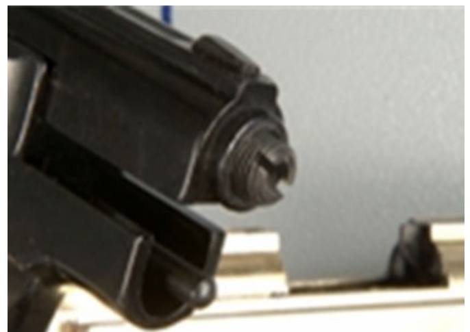
FIG. 5—Removable partial obstruction in the barrel.
