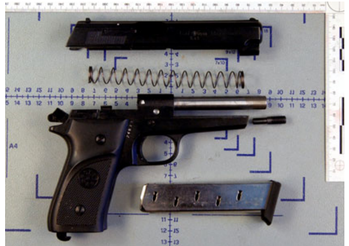
FIG. 9—Mounting a replacement barrel to the blank pistol.
