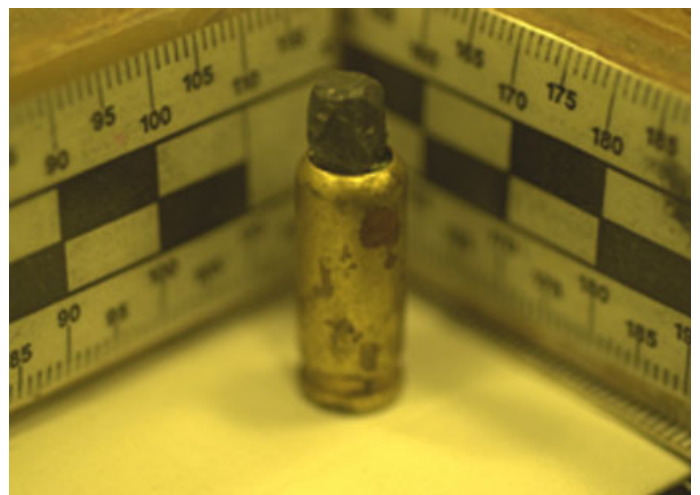
FIG. 7—Modified blank cartridges fitted with a larger spherical buckshot and an improvised projectile.
